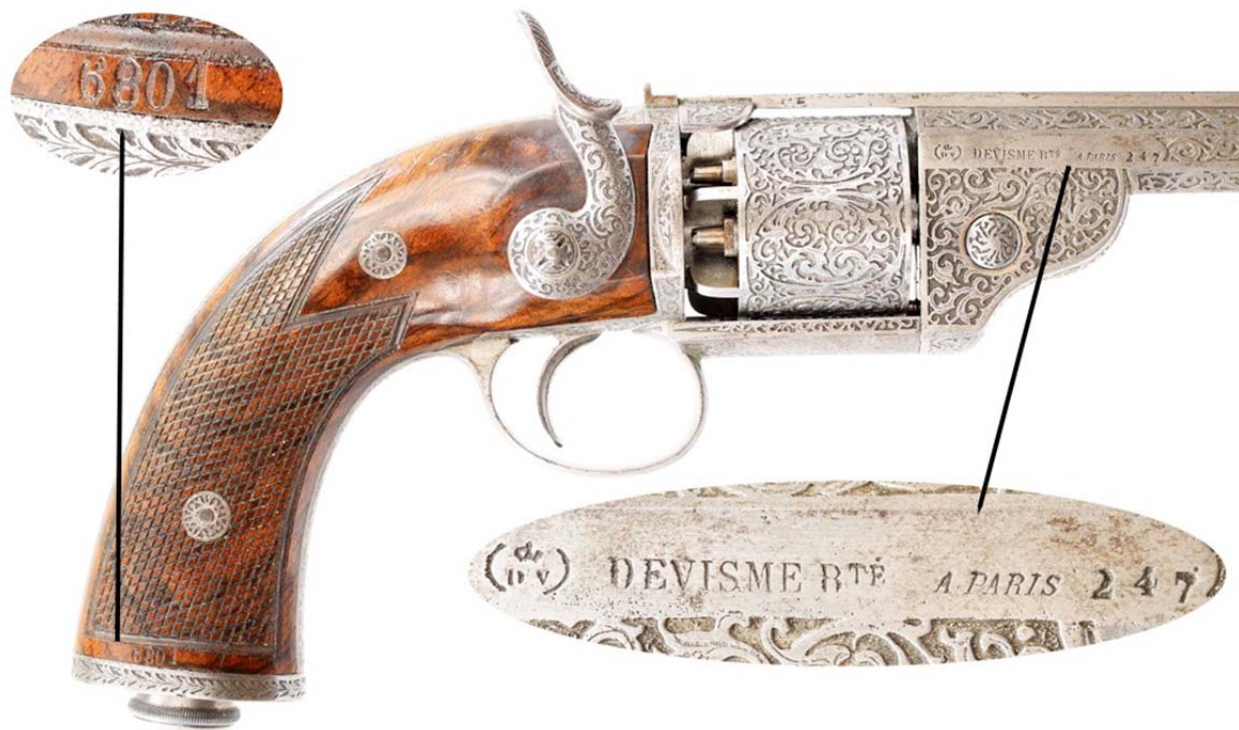
Fig. 7 – Close-up of the Devisme revolver showing the beautiful engraving and high-grade wood of the grips. Note the serial number on the right grip, and the maker's name, trademark and assembly number stamped on the right barrel flat.
