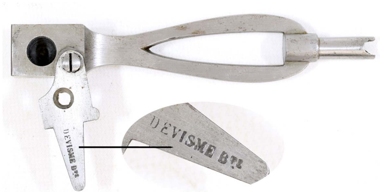
Fig. 11 - Combination bullet mold and cone wrench found in the case. Note the manufacturer's mark "DEVISME BTE."
