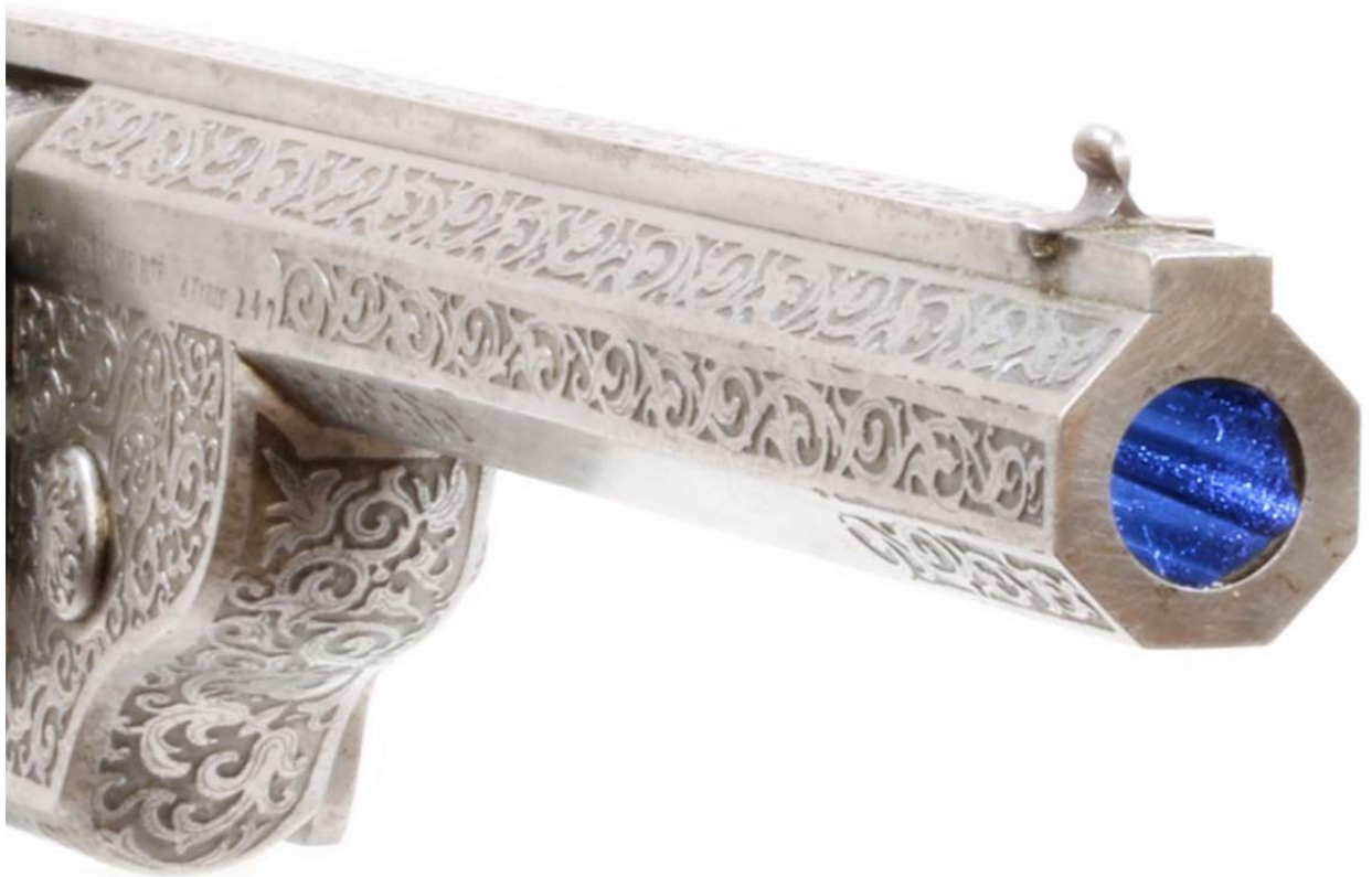
Fig. 9 – Devisme revolver. Close-up of the barrel, muzzle and front sight. The beautiful floral engraving that covers 80-90% of the gun is crisp and sharp, as is the rifling in the bore.
